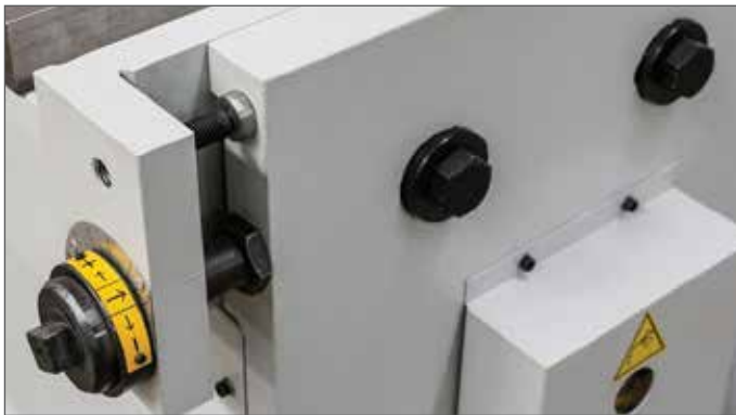
» Rigid frame and easy blade gap setting
